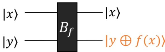
$$\boxed{B_f} : \underbrace{|x\rangle|y\rangle}_{\text{Input}} \mapsto |x\rangle \underbrace{|y \oplus f(x)\rangle}_{\text{Output}}$$
